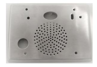
The High Security Steel Cover Plate (R5HSSCP-2) is a 3 gang, .050", stainless steel plate, designed to protect the R5 Staff Station when used in psychiatric wards and other high security hospital areas. The R5HSSCP-2 allows access to, and operation of, the station's call and cancel switches. The R5 Staff Station plastic cover plate is used with the R5HSSCP-2 and must have pass-through holes drilled for the four mounting screws. TheR5KLS-4 is not used with this plate configuration.
