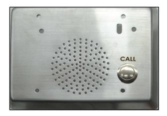
The High Security Steel Cover Plate (R5HSSCP-1) is a 3 gang, .050", stainless steel plate, designed to protect the R5 Staff Station (353101) when used in psychiatric wards and other high security hospital areas. The plate incorporates a vandal resistant dry contact switch which is used in conjunction with the R5KLS and is used to initiate a call from the room. When using the R5HSSCP-1, the R5 Staff Station plastic cover plate is not installed.
